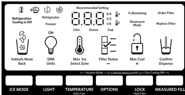
**IMPORTANT:** The display screen on the dispenser control panel will turn off automatically and enter “sleep” mode when the control buttons and dispenser paddles have not been used for 2 minutes or more. Press any control button to reactivate the display screen. The home screen will appear as shown.
