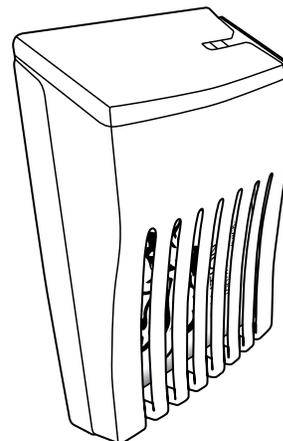
2. Open the housing by pulling up and out on the back.
