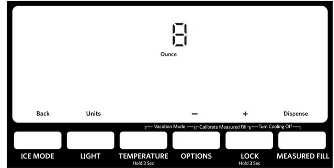
Press ICE MODE, under Back, to manually turn off the Measured Fill feature and return to the home screen.
