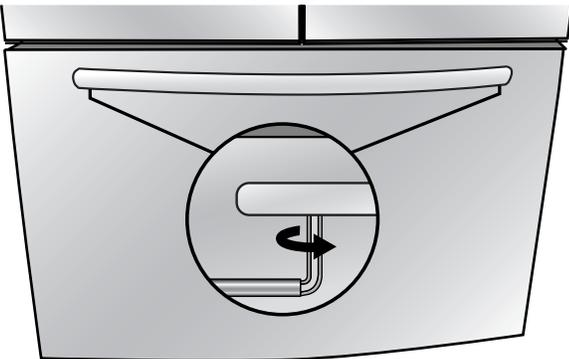
12. Using a left to right motion tighten the setscrew a quarter-turn at a time just until it begins to contact the shoulder screw. Do not fully tighten.
