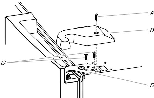
A. Top hinge cover screw      C.  $\frac{3}{16}$ " Internal hex head screws
