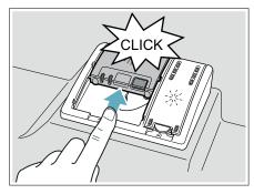
The detergent dispenser will open automatically at the ideal time for the set cycle. The powder or liquid detergent is distributed in the appliance and is dissolved, detergent tabs will fall into the detergent tab tray 24 where it dissolves during the cycle.
