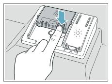
When using detergent tabs, lay them such that they do not come in contact with the cover, insert a detergent tab flat, not on its side.
