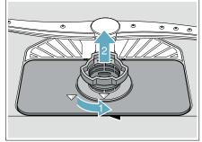
2. Remove the microfilter from the fine filter for easier cleaning.
