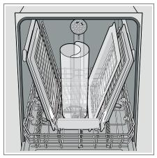
Note: Keep the vent hole 25 on the tub's left side clear by placing tall items such as plastic cutting boards and tall baking sheets on the lower rack's right side or center.
