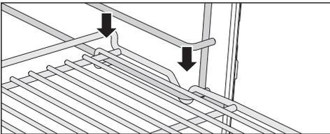
Always slide the Wire Rack into the rails of the side racks with the catches facing down.
